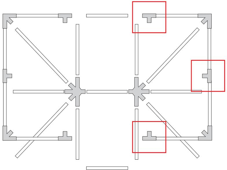
3. For the 40-foot side, slide each end of a (9'4") **Side Eave Bar** into the eave connector openings of the **Mid-Leg Rafter Fittings**, connecting both ends. Be sure the snap buttons engage. (Repeat for structures longer than 40') You should now have a completed eave section.
