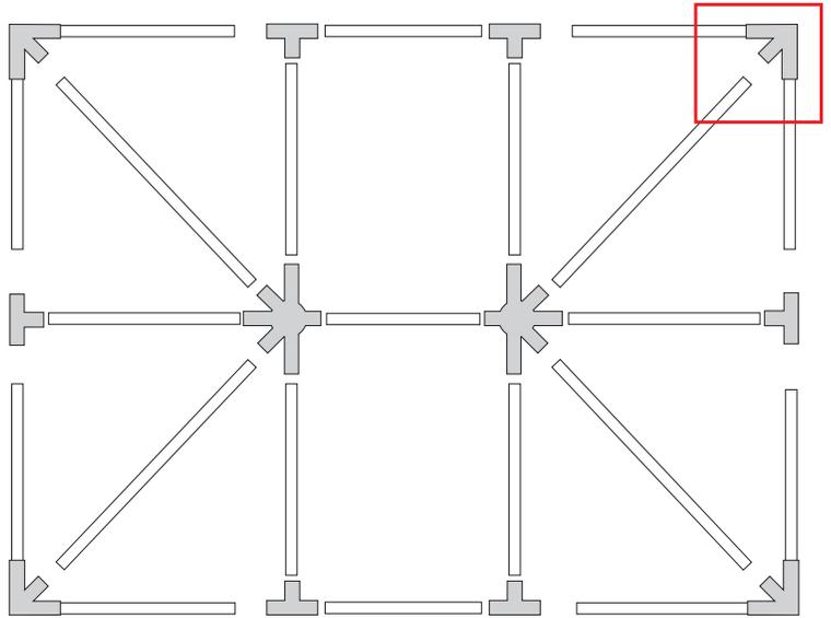
2. Then attach the other end of the **Side Eave Bars** to the eave connector opening of a **Mid-Leg Rafter Fitting** until the snap buttons engage. Be sure the rafter connector opening of the Mid-Leg Rafter Fitting is pointing inwards and the leg connector opening is pointing downwards. On the 30-foot side, there will only be one Mid-Leg Rafter Fitting that connects both Side Eave Bars.
