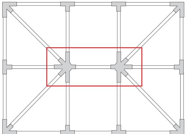
For structures longer than 40', connect the end 9'4" **Top Bars** to a **Top Extension Fitting**. Connect additional 9'4" **Top Bars** between the Top Extension Fittings and the opposite end 6-Way Crown Fitting. One at a time, insert a (16'1/4") **Mid-Rafter** to a **Mid-Leg/Rafter Fitting** until the snap button engages and connect the other end to the **Top Extension Fitting(s)** until the snap button engages.
